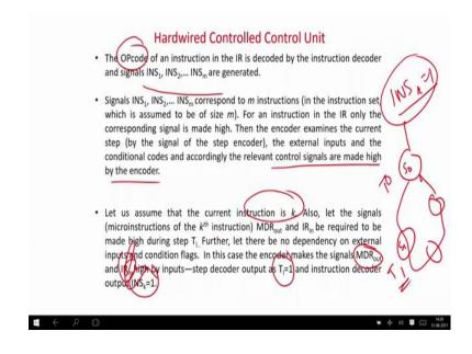
The opcode will actually generate signals  $I_1$  to  $I_m$ . So, if there are m signals based on opcode any one of them will be high and that will actually invoke the corresponding finite state machine. Correspondingly then the decoder examines the signal and accordingly the relevant control signals are made high by the encoder. In fact, actually it will select a corresponding finite state machine.
