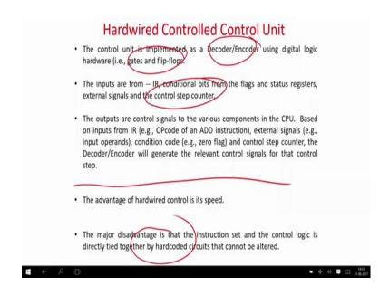
And then basically what happens we will finally have a decoder encoder and series of flip flops which will design the basic circuit which will take all this inputs and generate the corresponding output signals and in the proper sequence of steps of a finite state machine. So, it's a finite state machine based synthesis you have to run as I again repeating in the inputs are IR, condition bits flags, status registers, and basically your control step counter.
