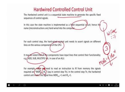
So, basically whatever I told you can read through over this slide it says that hardwired control unit is a sequential state machine; that is the finite state machine which will generate the sequence of controls.
